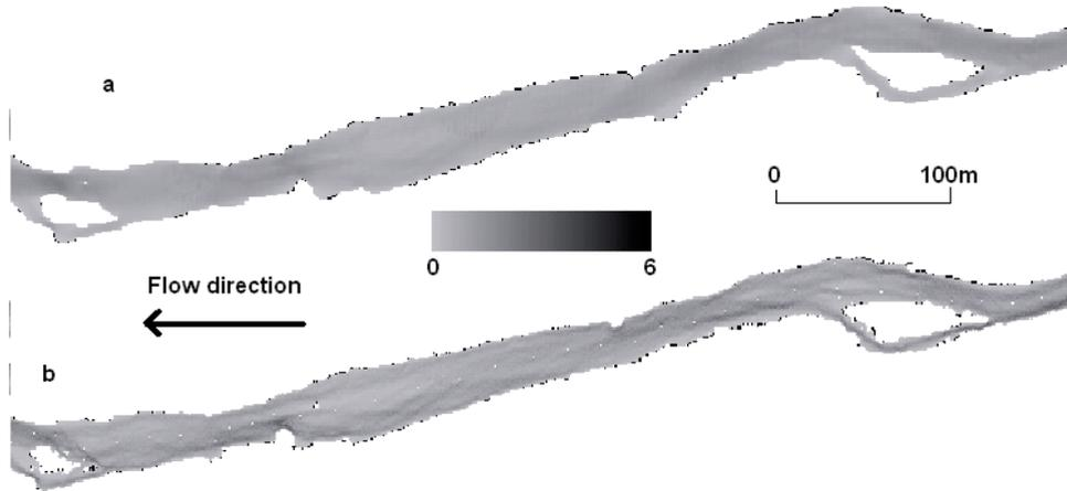
**Figure 3.** unit discharge generated for the sub reach of Walnut Gulch (Figure 1) using: (a) DELFT-3D flow (shallow water equations); (b) reduced complexity scheme. Total discharge  $20\text{m}^3\text{s}^{-1}$ .
