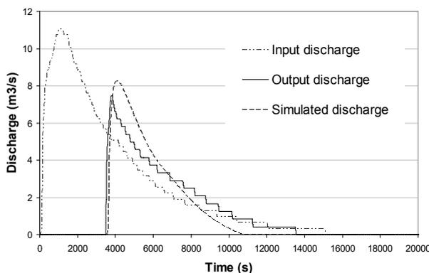
**Figure 2.** Observed and Simulated Hydrographs for the flow event on the 10/8/2006.
