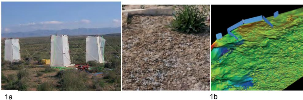
Figure 1.- 1a: the three rainfall simulators. 1b: open plot over a cyanobacteria-dominated crust and DEM of this plot.
