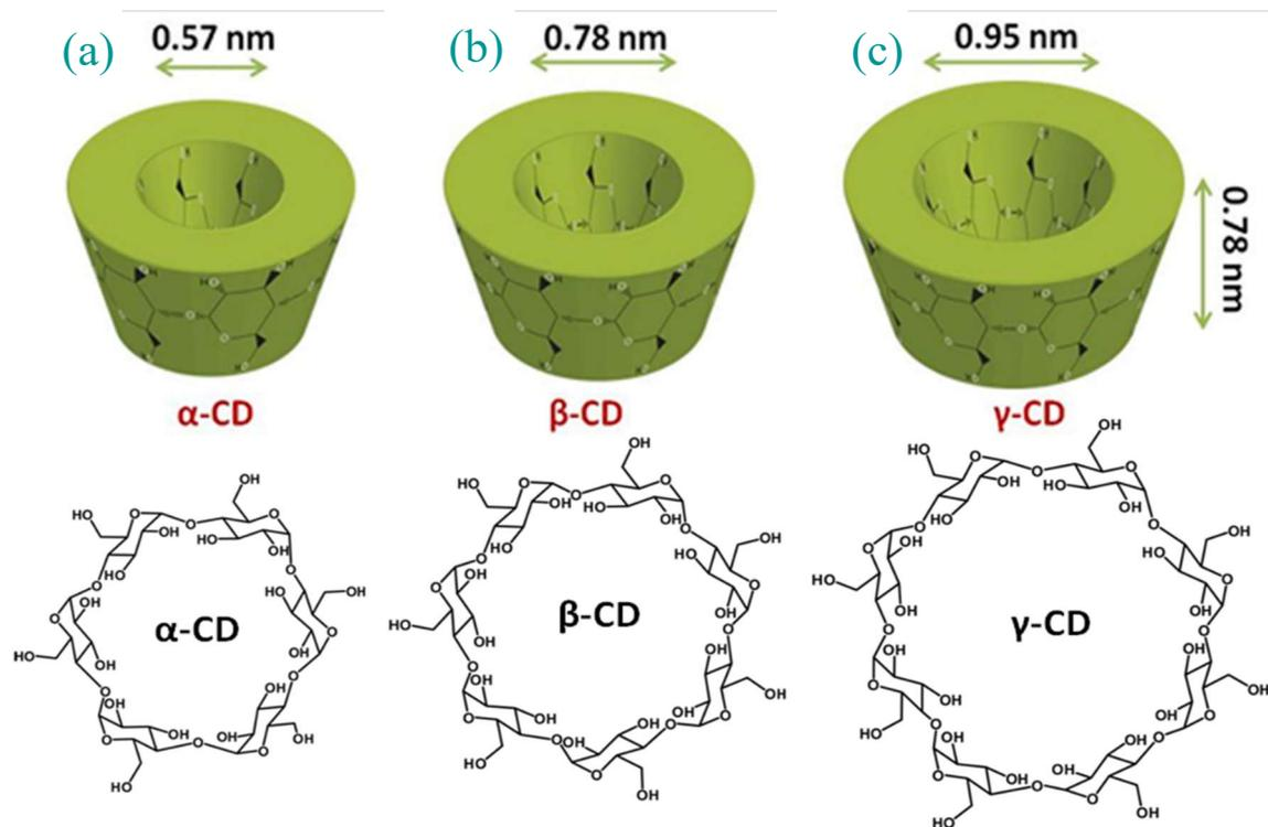
**Figure 7.** The molecular structure of different cyclodextrins (CDs): (a)  $\alpha$ -CD, (b)  $\beta$ -CD, and (c)  $\gamma$ -CD (Celebioglu *et al.*, 2017).
