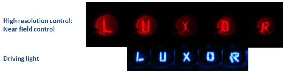
Fig. 3: example of high resolution near field projected images (top row) obtained by the illumination driving pattern in the bottom row, showing the name of our Lab.
