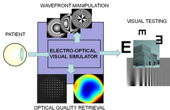
Fig. 1. Schematic diagram showing the operation of the Visual Simulator in white light
