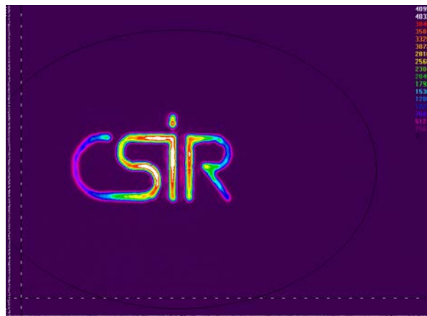
Fig. 3. SLMs have the advantage that arbitrary complex amplitude modulation can be executed even with a phase-only device.
