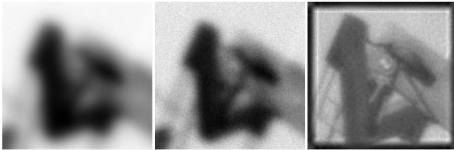
Fig. 1. Imaging at the horizontal path; reconstruction from 100 frames. Average (left), sharpest (center) and reconstructed (right) frames.
