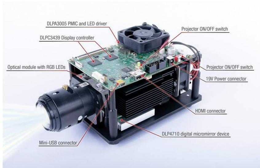
FIGURE 2.26: Stimulus projector - DLP4710EVM. For using in the AOVS, the projector lens was taken off, exposing internal DMD array. Source: ti.com
