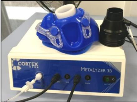
A blue and white gas analyzer device with a blue breathing mask on top. The front panel has 'CORTEX' and 'METALYZER 3B' printed on it. There are several ports and a power button on the front. |
