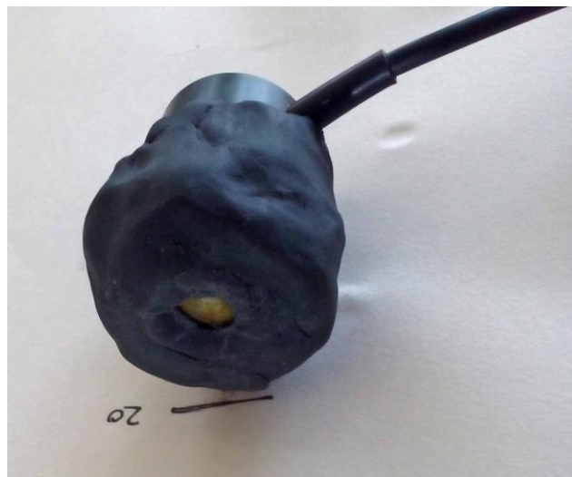
Fig. 3. Photoradiometer probe covered with the handmade mould used to evaluate the light transmitted by the fruit pericarp of Posidonia oceanica within the gradient of light intensity. In this image, the probe, with the fruit pericarp coupled inside it, was situated 20 cm from the light source.
