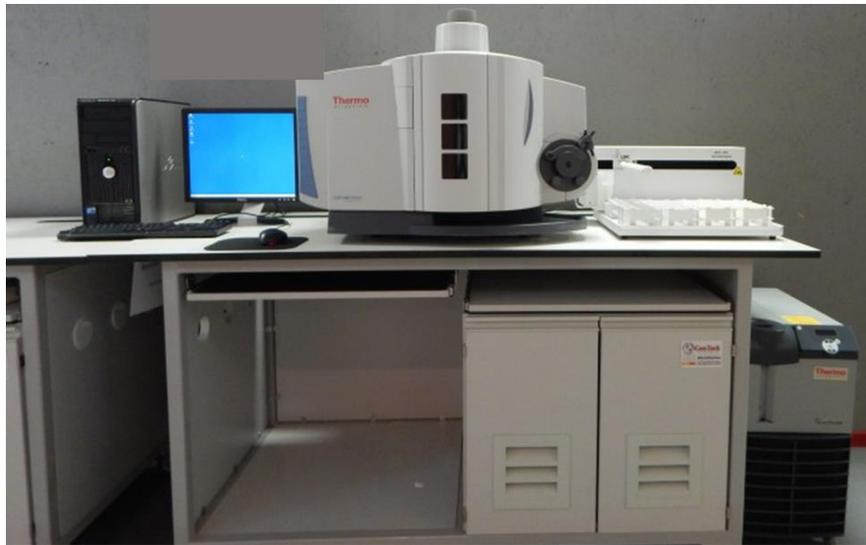
**Figure 10.** ICP-OES, Thermo ICAP 6000 SERIES, ThermoFisher Scientific)
