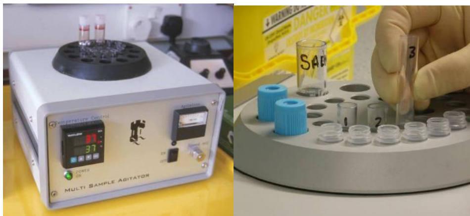
Figura 26. MSA (Multi Sample Agitator, University of Nottingham).
