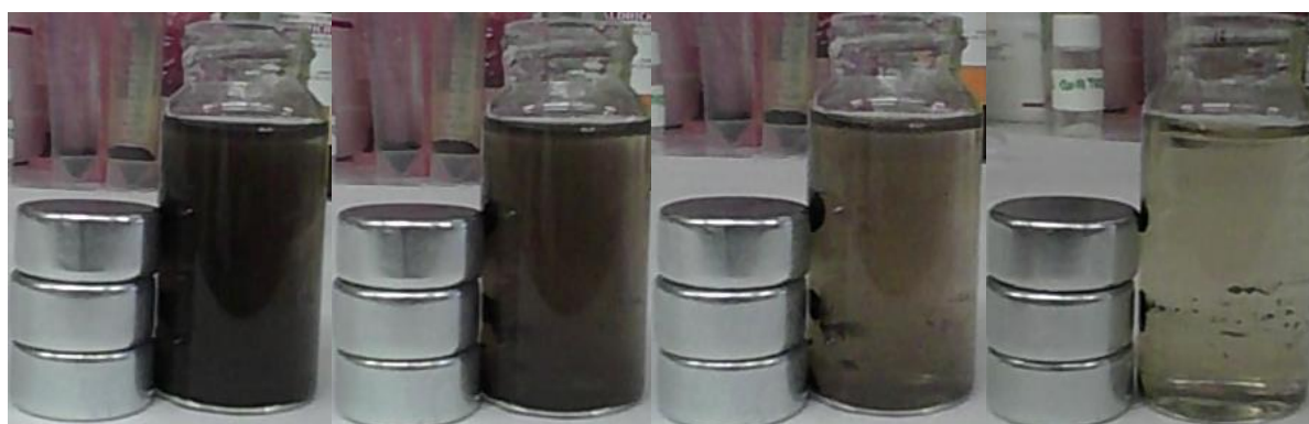
Fig 7: Images of the magnetic epoxy-CLEAs remove from the reaction medium with a neodymium magnet.
