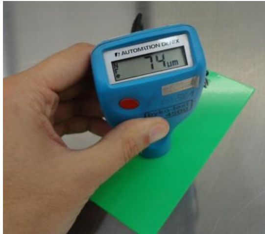
Figure IV.10. Thickness gauge (BYK Gardner, Byko-test 4500).
