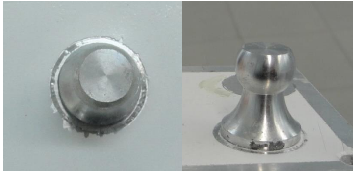
Figure IV.21. Dolly glued on powder coatings.
