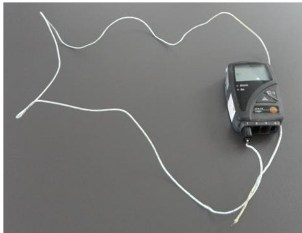
Figure IV.3. Logger 177. T4 testo: temperature controller.
