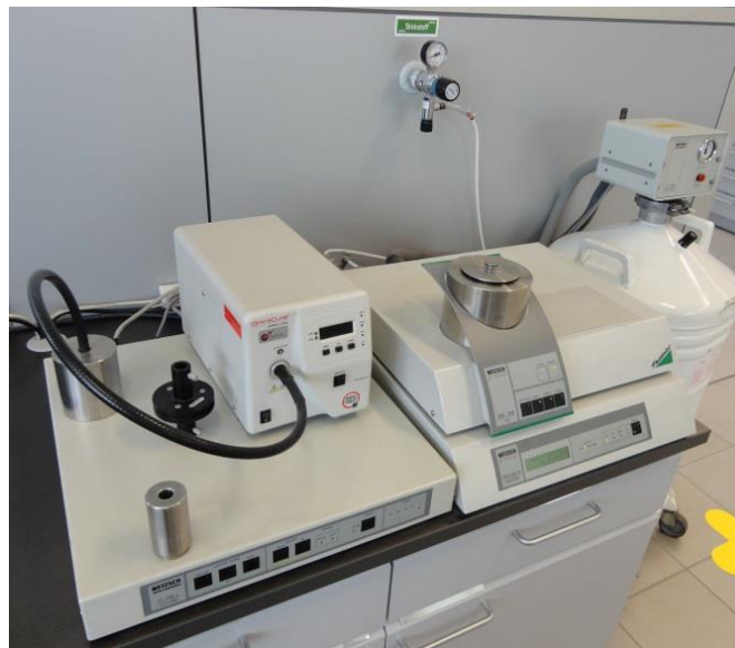
Figure IV.1. DSC Machine: NETZSCH DSC 204.
