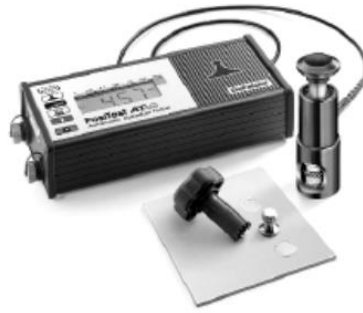
Figure IV.4. Pull-off test machine: PosiTest®.
