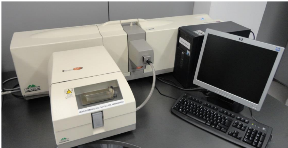
Figure IV.11. Particle size analyzer: Mastersizer 2000/ Scirocco 2000.
