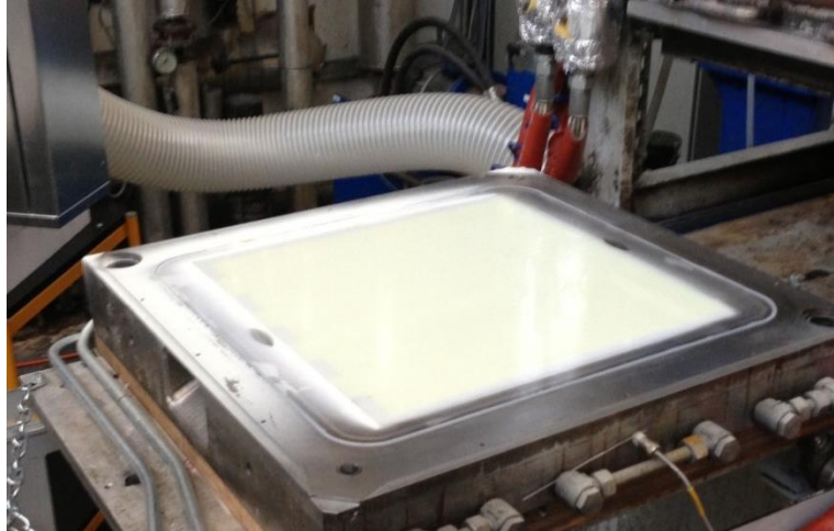
Figure III.20. Coated mold by powder coatings.
