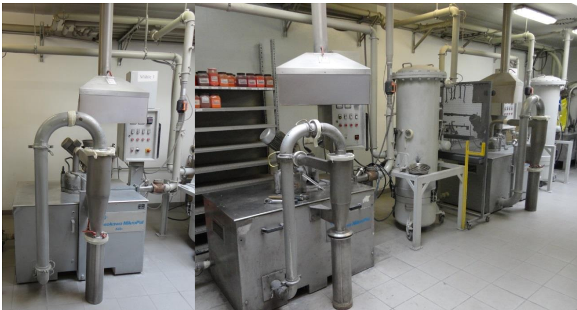
Figure IV.2. Grinding Mill: Hosokawa Mikro Pul Köln ACM 2L.
