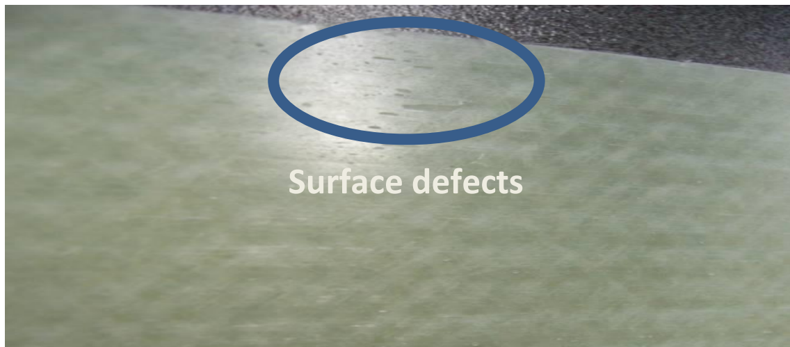
Figure III.19. Composite with surface defects.
