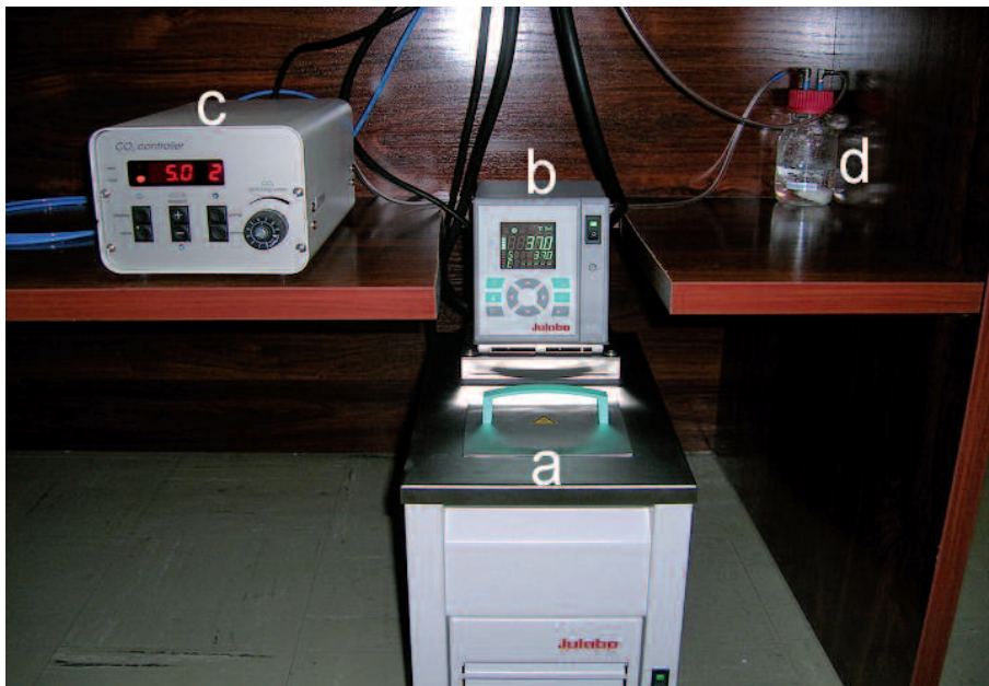
Fig. 2. Water temperature was regulated with the thermostat, controlling it by means of an electronic feedback system (Julabo F25). The thermostat is formed by the water reservoir and pump (a), the electronic feedback and temperature measurement system (b). c. CO 2 controller (PeCon). Cells were maintained in this way at a stable temperature of 37.0 \pm 0.1^\circ\text{C} , within an accurately controlled 5% CO 2 atmosphere, humidified after passing the circulating water through a sterile water flask (d).
