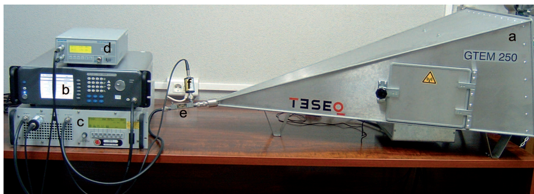
Fig. 5. Experimental irradiation set-up. a. Gigahertz Transversal Electromagnetic Mode Cell (GTEM-cell). b. MW functions generator. c. Travelling wave tube power amplifier. d. Diode bridge power meter. e. Directional coupler. f. 50 \Omega field probe for reflected EM wave power measurement.
