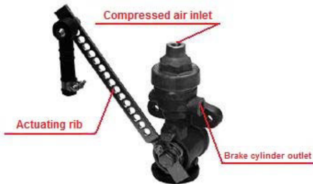
Fig. 2. Mechanical Load Sensing Valve (LSV) [5].
