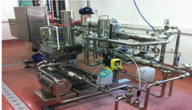
Figure 5.14 Food industry pilot plant for pH control experiments.
