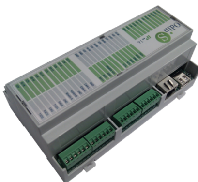
Figure 7. Home automation module developed.
