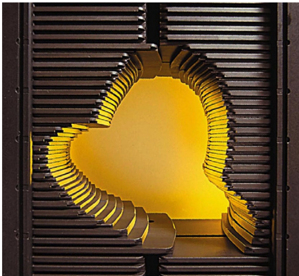
Figura 4. Colimador multiláminas (Bortfeld, 2006).
