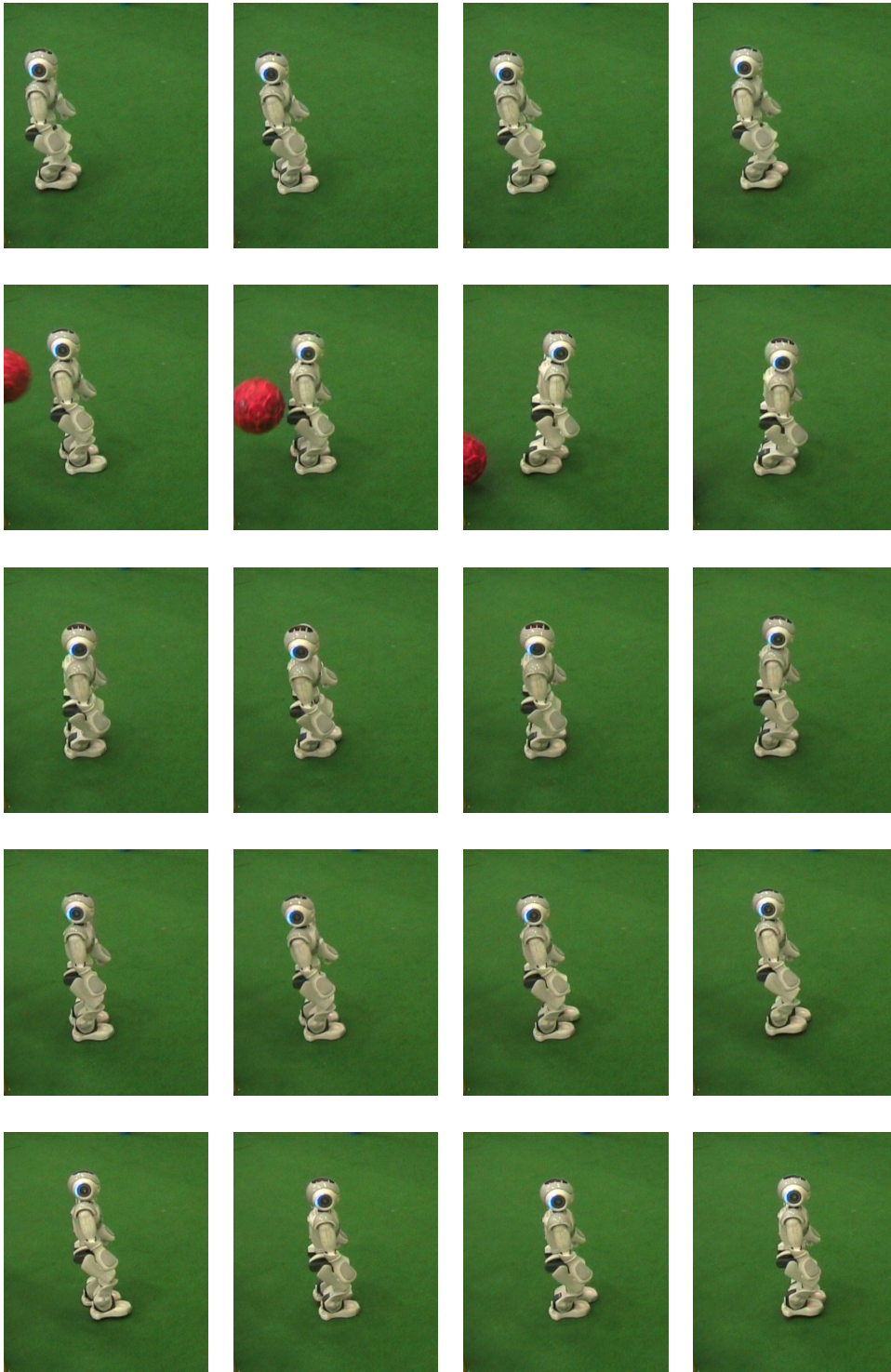
Figure 6.7: Sagittal disturbance rejection during forward walking.
