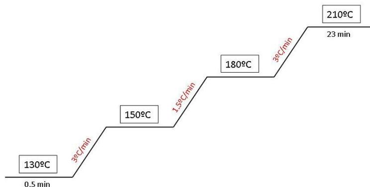
Figure 6: Gas chromatography analysis conditions with respect to the program of temperatures used for fatty acids methyl esters quantification.
