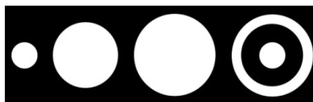
Figure 8.2: Pupils for which optical quality through-focus was predicted. The small aperture pupil of 1.6 mm, a natural photopic pupil of 4 mm, a natural scotopic pupil of 5 mm, and the annulus pupil of 5 mm (inner inlay diameter 1.6 mm, outer inlay diameter 3.8 mm).
