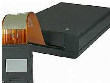
Figure 2.3: Photo of the reflective liquid crystal on silicon spatial light modulator.
