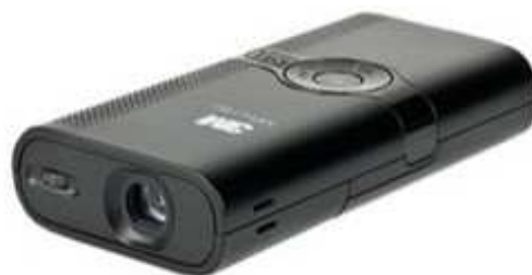
Figure 2.15: Pocket projector which was converted into a microdisplay by removing the zoom lens.
