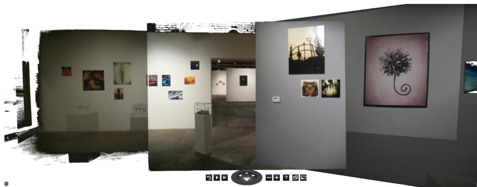
Figure 1.4: Navigable image mosaic, generated with with Photosynth [Labs, 2012] from pictures captured inside an art gallery. Photosynth is an on-line application based on the Phototourism project for SfM reconstruction [Snavely, Seitz and Szeliski, 2006]. The application renders on an image mosaic the approximate visual appearance of the scene, as seen from a given view point. The user can change this view point using the interface to navigate through the scene in a simulated virtual presence.
