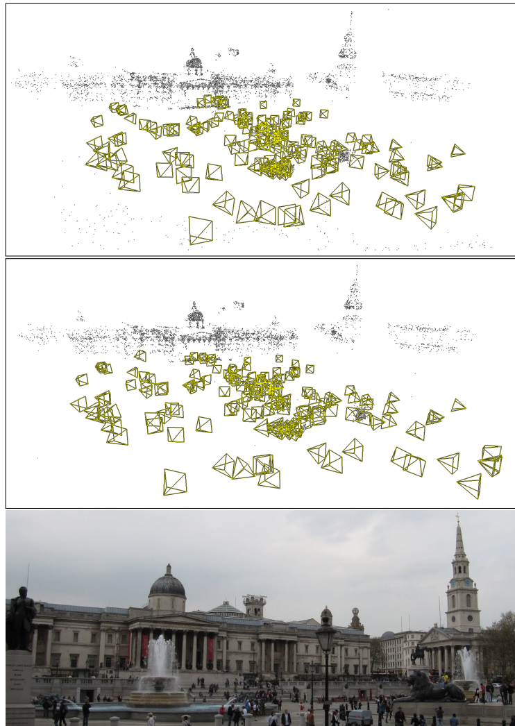
Figure 5.17: Camera poses and detail of the sparse scene structure obtained from the dataset trafilgar-161 , using the following methods: Top: correction of the camera poses contained in the dataset with GEA, and re-estimation of the structure with the linear triangulation. Middle: incremental motion estimation and the linear structure triangulation from the pairwise matching information contained in the dataset. Bottom: picture from the original scene (Author: https://ssl.panoramio.com/user/3029536 ).
