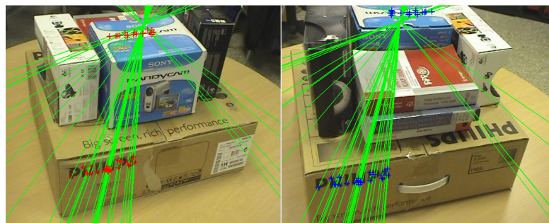
Figure 4.5: Epipolar lines for the mismatches shown in figure 4.4 which were obtained with an incorrect epipolar geometry. In this case the image features (red and blue crosses) are sufficiently close to the epipolar lines (green lines) obtained with an incorrect epipolar geometry. This misleads the sample consensus search into considering the mismatches and the epipolar geometry as valid.
