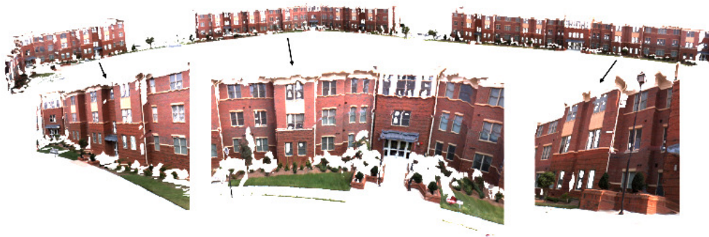
Figure 1.1: 3D model of the facades in a street side, obtained on-line from a moving vehicle with the system described at [Akbarzadeh et al., 2006]. The reconstruction application runs on an on-board computer, equipped with a powerful Graphical Processing Units (GPU's), and obtains a simplified 3D model of the street, consisting on planar surfaces detected at the building facades.
