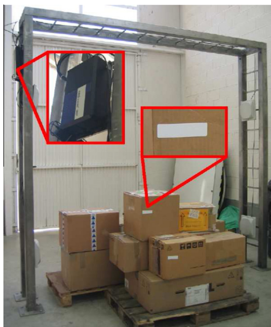
Fig. 6. RFID-UHF reader and antenna rack of the trailer, mounted for testing purposes in laboratory.
