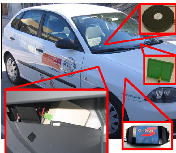
Fig. 12. Integration of the system in a real vehicle fleet. The emphasized elements are listed in clockwise order: the GPS/GPRS-UMTS and RFID-HF antennas, the OBD-II reader, and the OBU module.
