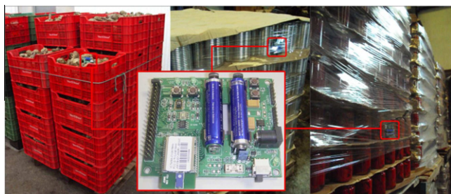
Fig. 7. Integration of the ZigBee RFD node (marked in red), with humidity, temperature and light sensors in three supply chain stages. Left: sensors attached to the artichokes immediately after being harvested from the market garden. Middle: sensors affixed to a pallet of tinned peaches. Right: sensors affixed to a pallet of pepper jars. (For interpretation of reference to colors in this figure legend, the reader is referred to the web version of this article.)
