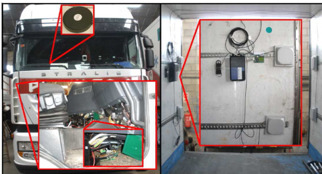
Fig. 10. Integration of the system prototype in a truck. On the left the cabin elements are seen as integrated into the truck dashboard: the GPS/GPRS antenna (up) and OBU (down). On the right the deployment in the trailer. The RFID antennas have been installed around the rear door, near the RFID-UHF reader and the TCU.
