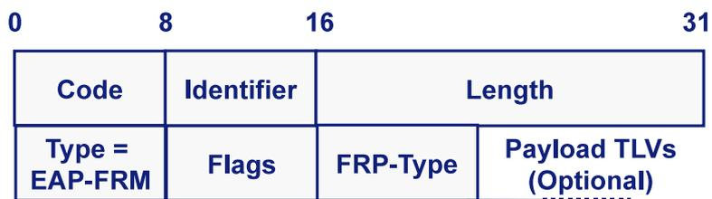
Figure 3.4: EAP Fast Re-authentication Method (EAP-FRM)
