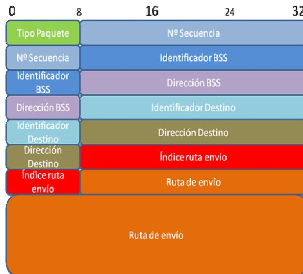
FIGURA 14 MENSAJE REGISTER REPLY
