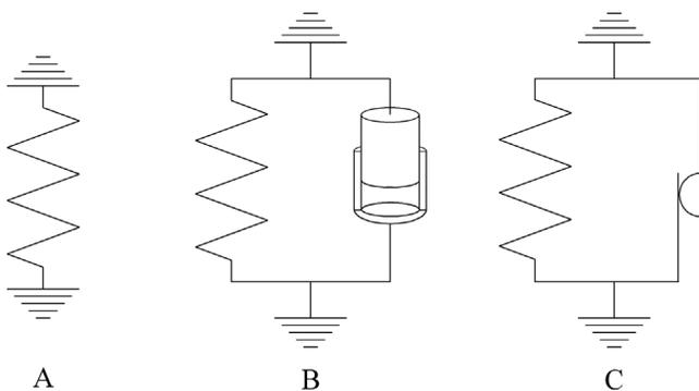
**Fig. 2.** Diagram of three bodies with different properties. **A:** Elastic body, spring. **B:** Viscoelastic body, spring connected in parallel to a dashpot. **C:** Protoelastic body, spring connected in parallel to a dry friction element.
