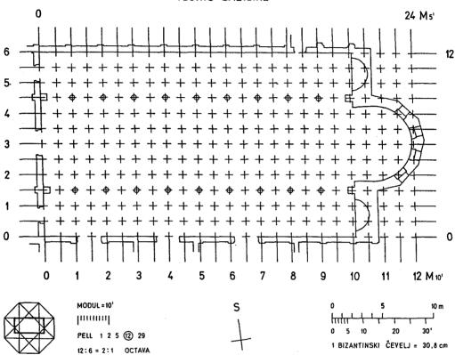
ILLUSTRATION 5. The distorted plan of the Basilica on the planning grid. The module is 10 podes long.
