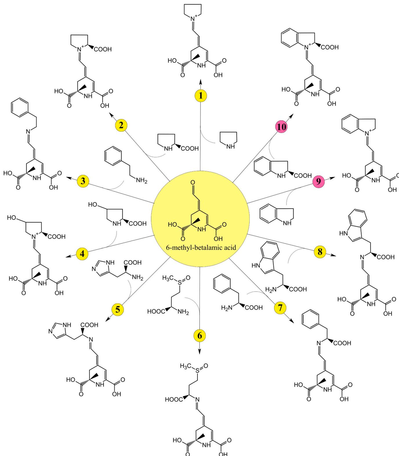
**Fig. 5.** Scheme representing the reaction between 6-methyl-betalamic acid and (1) pyrrolidine, (2) proline, (3) phenylethylamine, (4) hydroxyproline, (5) histidine, (6) methionine sulfoxide, (7) phenylalanine, (8) tryptophan, (9) indoline, and (10) indoline COOH to yield methylated betalains.
