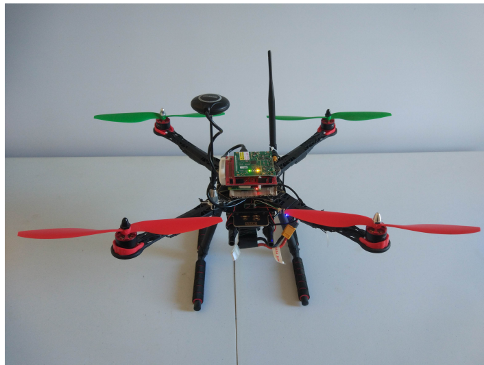
Figure 2. LoRa-drone gateway implementation used for testing.
