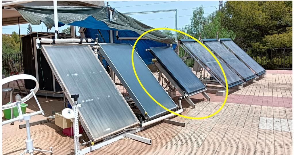
**Figure 2.** Solar collectors at the Solar Laboratory of the UMU. Conventional solar thermal collectors (left), PVT hybrid collector (centre) and vacuum tubes (right).
