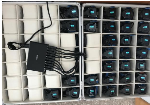
Fig. 3 – Box with smart bracelets plugged into the electrical power supply.
