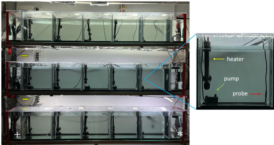
**Figure S1.** Photo of the three multi-chamber glass tanks built for investigating daily variation of thermal preference in fish. Each chamber is equipped with a mini water pump (green arrow), a thermostat resistance heater (yellow arrow) and a temperature probe (red arrow). In the right-extreme chambers of each multi-chamber tank (white asterisk), there
