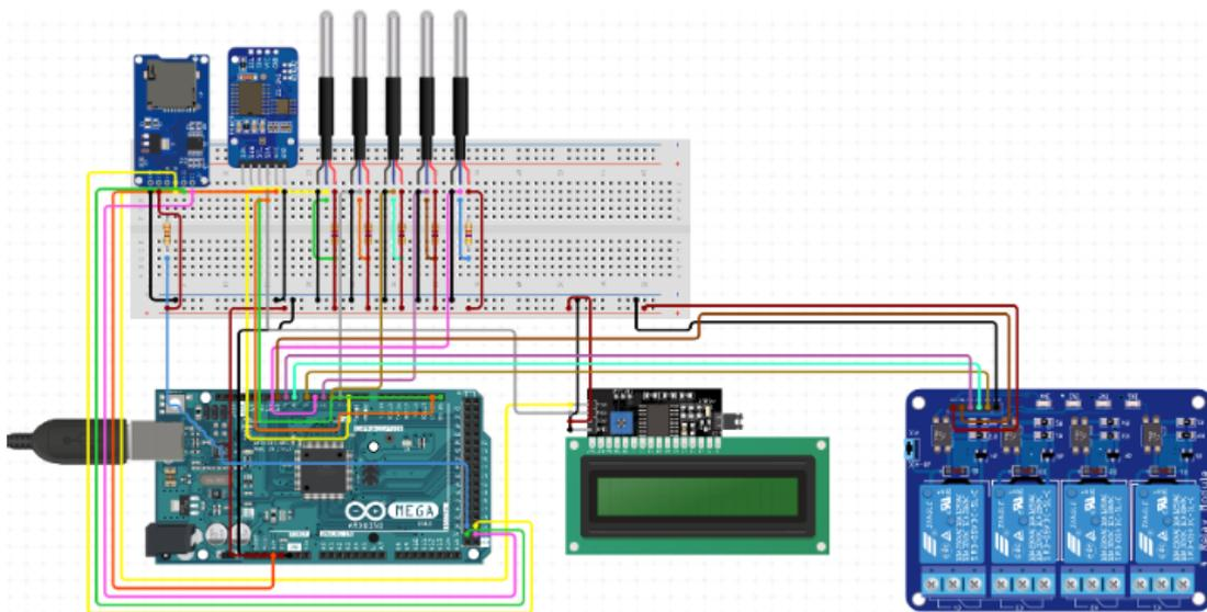
**Figure S3.** Arduino-based microcontroller circuit built to create the horizontal thermal gradient in the multi-chamber tank.
