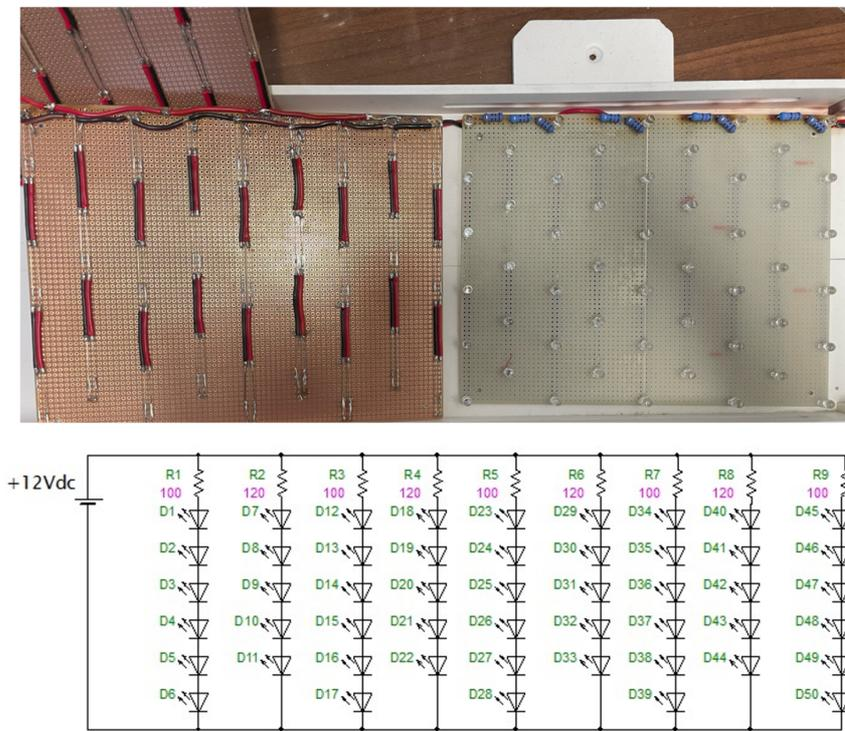
**Figure S2.** Photo and representative diagram of the circuit used to create infrared LED lamp. Each lamp presented 5 panel connected in series, where each panel consist in 50
