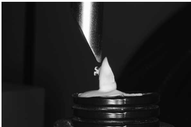
Figure 1. The sharp end of the rod incised in the area between the base and the wings of the bracket exerting a force parallel to the tooth surface in an incisal-apical direction.
