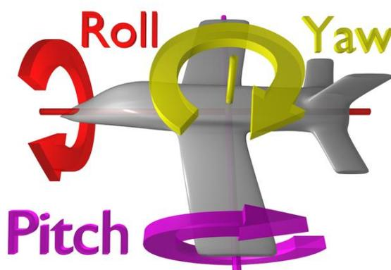
Figura 6.4: Yaw (Azimuth), Pitch y Roll
