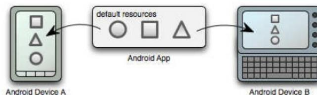
Figure 1. Two device configurations, both using default resources.
