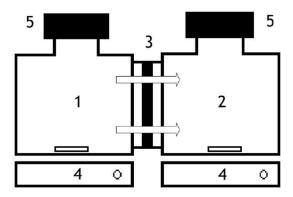
**Figure 1.** Diffusion cell discontinuous set-up used for experiments: (1) feed solution; (2) receiving solution; (3) PILIM; (4) magnetic stirrer; and (5) septum.
