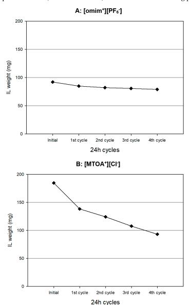
**Figure 3.** Profile of the weight losses of ionic liquid from PILIMs after each cycle in contact with the hydrochloric solution for different ionic liquids. (**A**)  $[omim^+][PF_6^-]/PVC$  (30/70) (**B**)  $[MTOA^+][Cl^-]/PVC$  (70/30).
