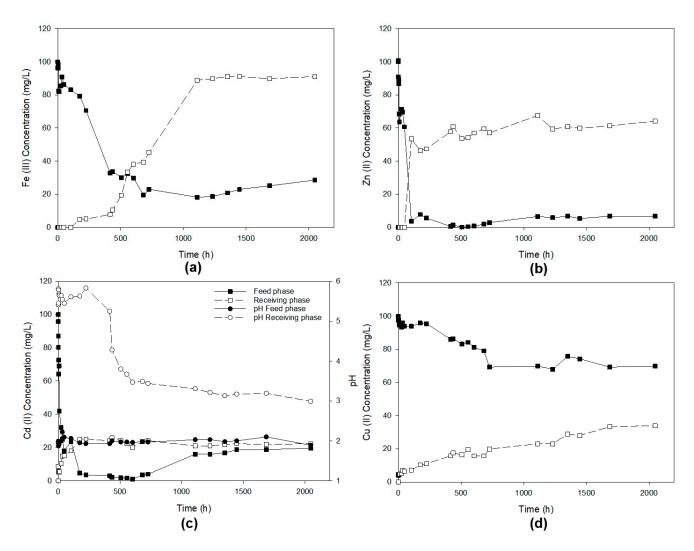
**Figure 5.** Metal ions concentrations and pH profiles in the feed and receiving phases in the transport of Fe(III) (**a**), Zn(II) (**b**), Cd(II) (**c**) and Cu(II) (**d**) through a PILIM based on [MTOA $^+$ ][Cl $^-$ ]/PVC whit 70% of IL. The feed phase was a mixture of the four metals ions (100 mg/L each) in HCl (1 M). The receiving phase was milli Q water at pH = 6.
