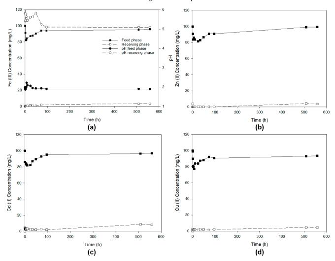
**Figure 4.** Metal ions concentrations and pH profiles (a) in the feed and receiving phases in the pertraction of Fe(III) (a), Zn(II) (b), Cd(II) (c) and Cu(II) (d) through a PILIM based on  $[omim^+][PF_6^-]/PVC$  with 30% of IL. The feed phase was a mixture of the four metal ions at 100 mg/L in HCl (1 M). The receiving phase was milliQ water at pH = 6.
