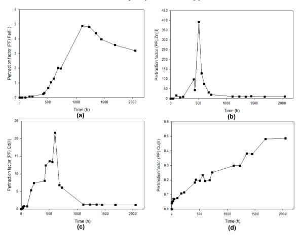
**Figure 7.** Profile of the pertraction factor (PF) of (a) Fe(III), (b) Zn(II), (c) Cd(II) and (d) Cu(II) using a PILIM based on [MTOA<sup>+</sup>][Cl<sup>-</sup>]/PVC whit 70% of IL. The feed phase is a mixture of the four metals ions (100 mg/L each) in HCl (1 M). The receiving phase was milliQ water at pH = 6.
