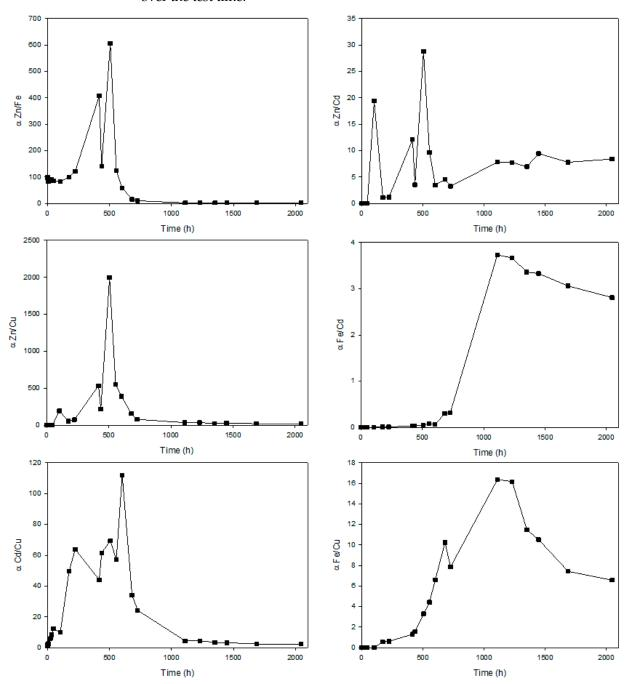
**Figure 8.** Profile of the separation factors for pairs between Zn(II)/Fe(III), Zn(II)/Cd(II), Zn(II)/Cu(II), Fe(III)/Cd(II), Cd(II)/Cu(II) and Fe(III)/Cu(II) using a PILIM based on [MTOA<sup>+</sup>][Cl<sup>-</sup>]/PVC whit 70% of IL. The feed phase consists of a mixture of the four metals ions (100 mg/L each) in HCl (1 M). The receiving phase was milliQ water at pH = 6.
