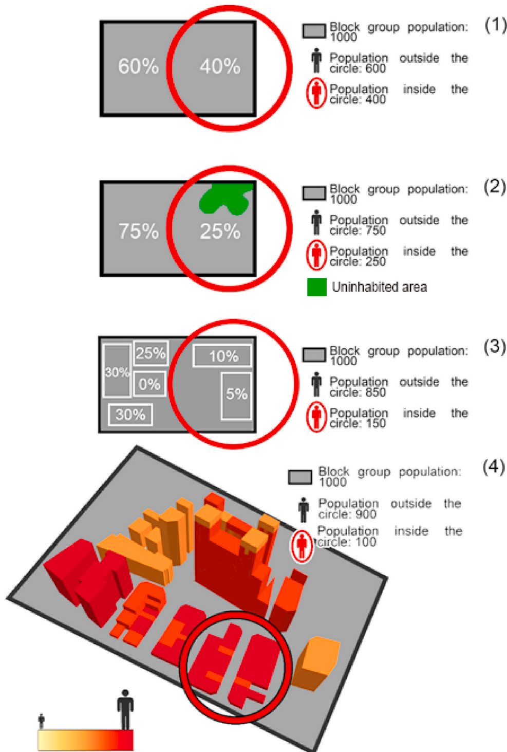
Fig. 1. Comparison of dasymetric methods: Areal Interpolation (1), Binary (2), CEDS (3) and Dasymetry Dash Flood (4). Methods 1, 2 and 3 were obtained from (Maantay et al., 2007). The red circle represents the exposed area.
