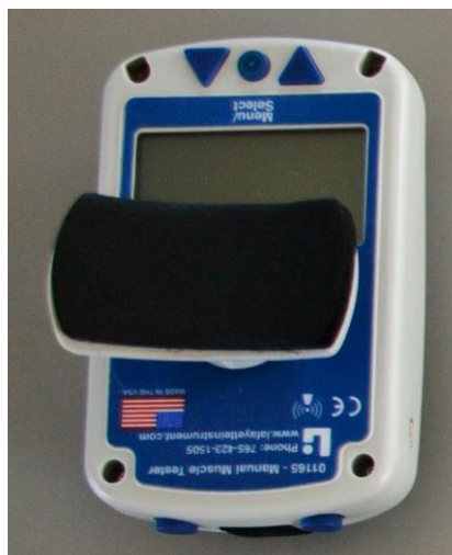
Figura 9: Dinamómetro Lafayette Manual Muscle Tester 01165
