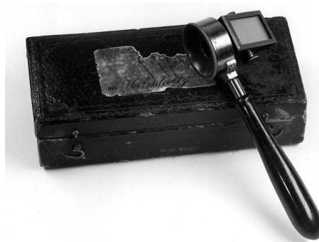
Figure 1.7. The early model of the direct ophthalmoscope was invented by Helmholtz in 1851 (Image adapted from [Keeler, 2002]).
