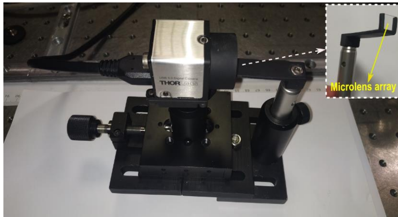
Figure 2.11. The arrangement of the HS sensor mounted on a precision stage. The microlens array in its 3D-printed holder is shown on the top right.
