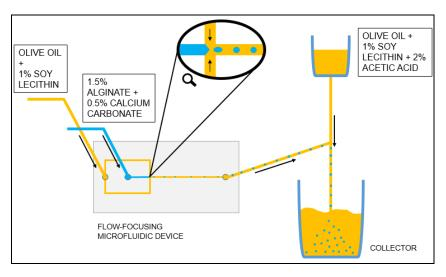
Fig. 1. Schematic representation of the flow-focusing microfluidic device.
