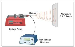
Fig. 1. Schematic representation of the electrospinning process.
