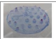
Fig. 1. Patterned hydrogel showing surface ridges.
