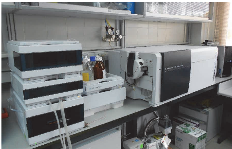
Figure 25: UPLC 1290 Infinity, Agilent Technologies, coupled to a 6460 Triple Quadrupole MS detection system
