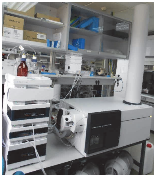
Figure 23: Agilent 1290 Infinity LC system coupled to the 6550 Accurate-Mass Quadrupole time-of-flight MS detection system.
