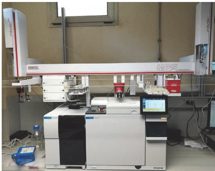
Figure 26: Agilent 7890A gas chromatograph system coupled to an Agilent 5975C mass selective detector.
