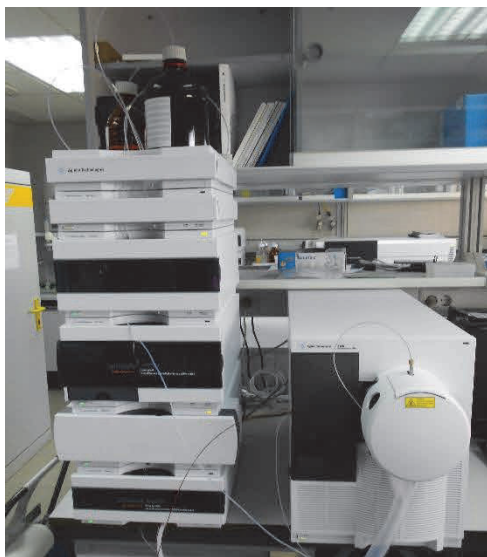
Figure 24: HPLC 1200 Series, Agilent Technologies coupled with a photodiode-array detector and single quadrupole MS detector (6120 Quadrupole, Agilent Technologies) in series.
