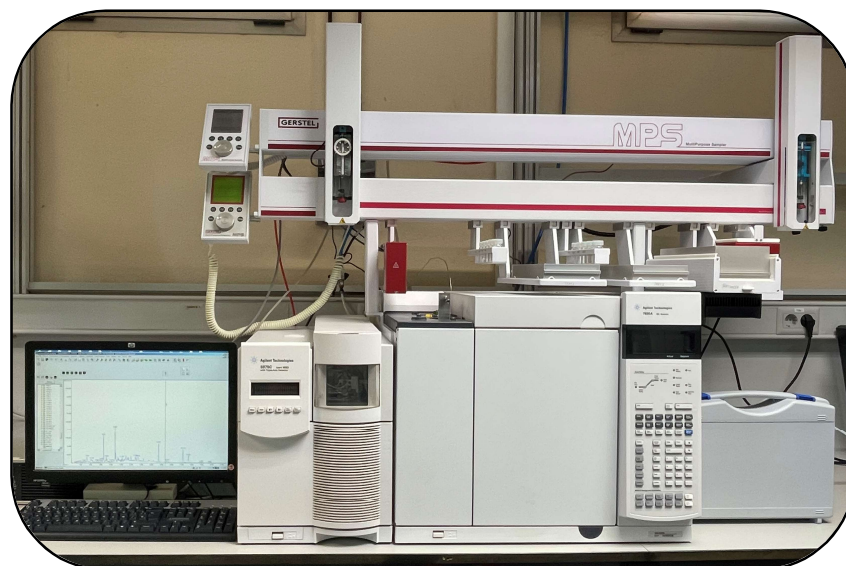
Fotografía 3.11. GC-MSD 5975C series inert MSD (Agilent).
