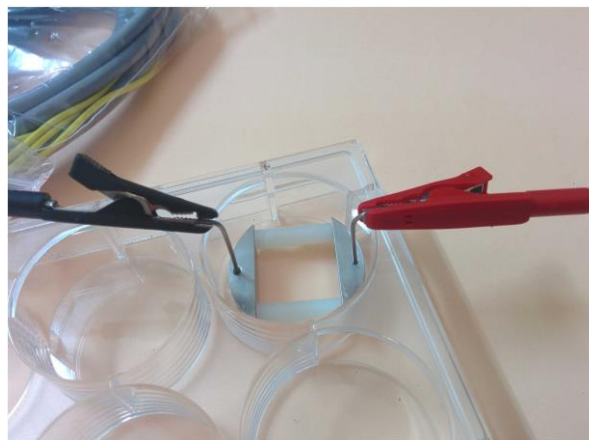
Figure 18. Device designed to apply galvanic current in 6-well plates. The two poles are separated by plastic spacers and generate a homogeneous and constant galvanic current through the well.
