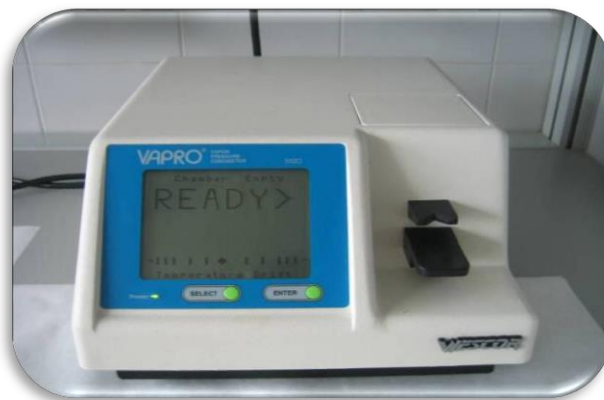
Picture 3. WESCOR 5520 vapor pressure osmometer (Wescor Inc., Logan, UT, USA).
