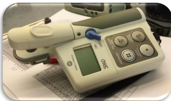
Picture 4. Minolta SPAD-502 chlorophyll meter (Konica Minolta Sensing Inc., Osaka, Japan) (left) and fluorimeter (IMAGING-PAM M-series, Heinz Walz, Effeltrich, Germany) (right).
