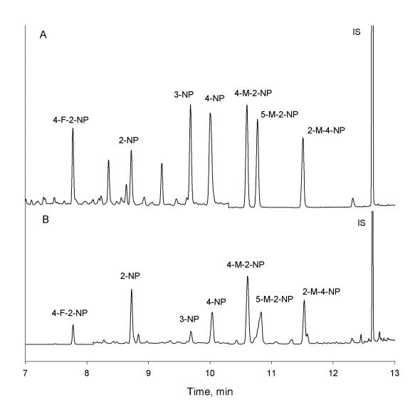
**Fig. 1.** Elution profile obtained with the optimized SBSE-TD-GC-MS procedure under SIM mode for a fortified water at 10 ng mL<sup>-1</sup> **(A)** and a fortified soil at 33 ng g<sup>-1</sup> **(B)** for each analyte.
