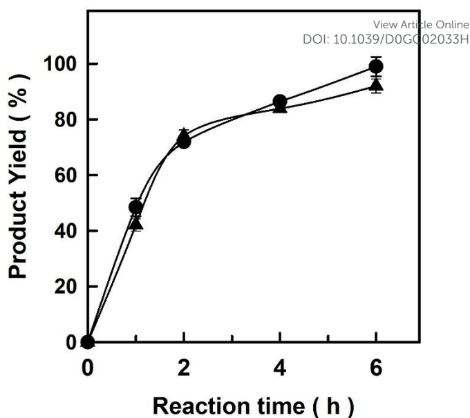
Figure 2. Yields obtained for the Novozym-435-catalysed synthesis of FASEs by the transesterification of triacylglycerides from linseed (●) or fish oil (▲) with solketal in 40% w/w [C 18 tma][NTf 2 ] at 60 °C.
