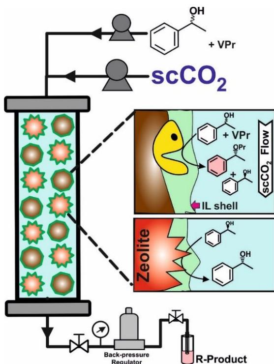
**Fig. 4.** Schematic representation of a SILP /  $scCO_2$  biphasic system used for the dynamic kinetic resolution (DKR) of *rac*-1-phenylethanol carried out by using vinyl propionate (VPr) as acyl donor, and the combined action of an immobilized lipase and an acidic zeolite as catalysts.<sup>83</sup>
