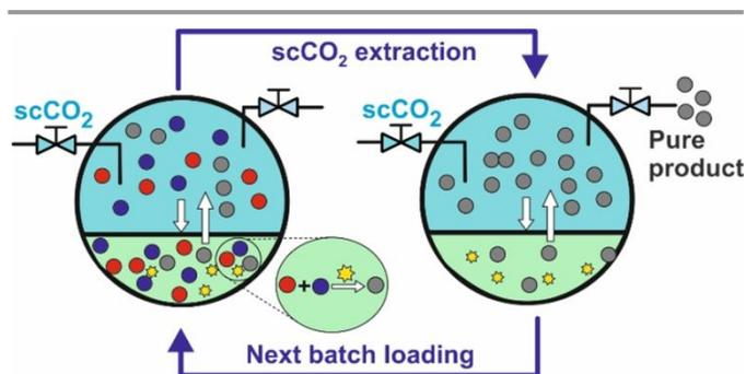
Fig. 3. General scheme for integrated reaction separation processes in IL/scCO<sub>2</sub> biphasic systems.
