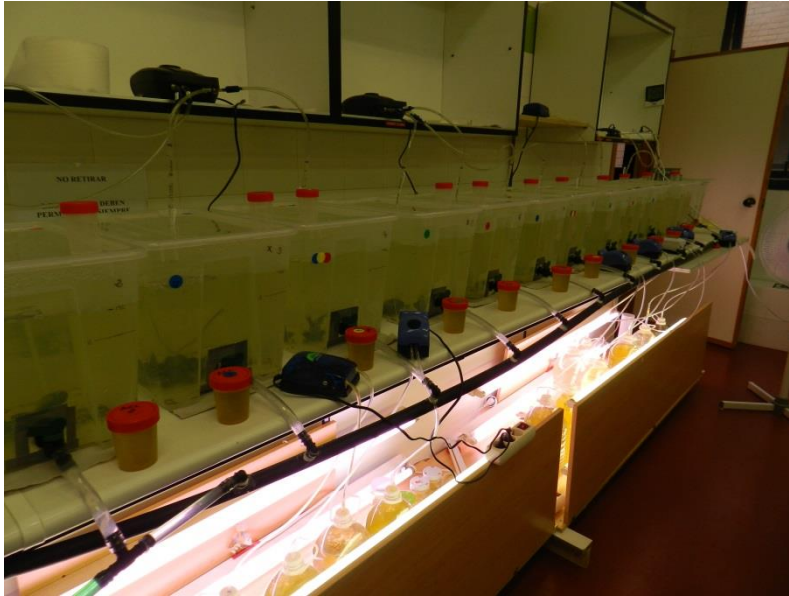
Figure 8. Mytilus galloprovincialis were exposure in tanks during seven days under controlled environmental conditions of pH, temperature, feeding, osmolarity and heavy metal concentration.
