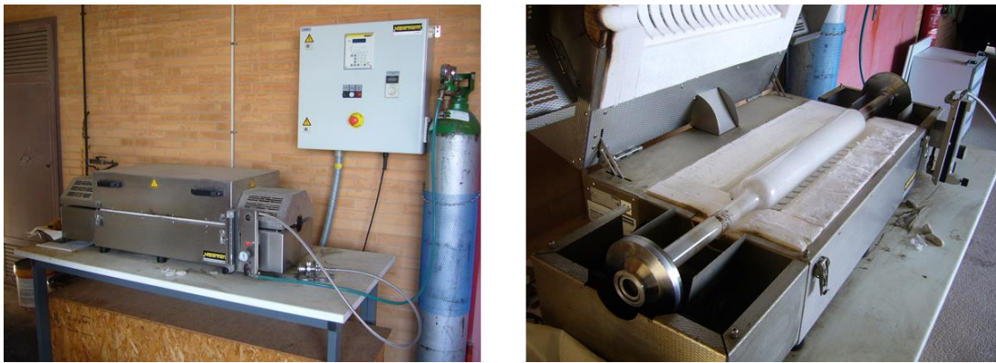
Figure A1. Pyrolyzer RSR-B 80/500/11, Nabertherm (Germany) used for the production of biochar at CEBAS-CSIC.
