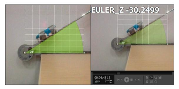
**Figure 1.** Procedure of Phase 1. The left image shows the inertial device attached to the goniometer, the position of the camera, and the automatic tracking function of the Kinovea calculating the angle. On the right, QÜIKO software automatically calculates the same angle.
